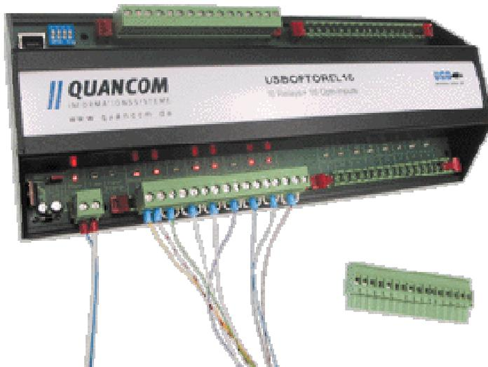
The QUANCOM® USBOPTOREL16 board has 16 opto inputs and 16 relays and is designed for industrial purposes. The relays are able to switch up to 1A / 15W. To switch higher capacity and voltage external relays are necessary. This is for example our QUANCOM® [MODSSR230](#) for 230V.
