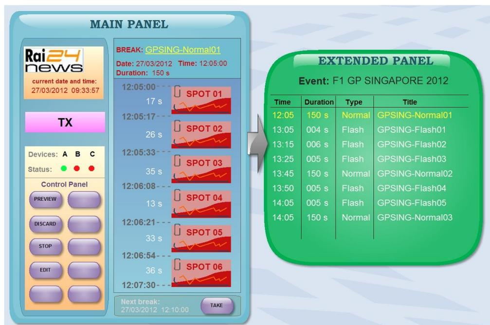
As shown in the figure above, each time a break is cued, it will be entirely loaded in the **main panel** and highlighted -in yellow- in the **extended panel**.
