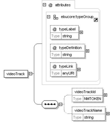
Figure 6: EBUCore videoTrack
